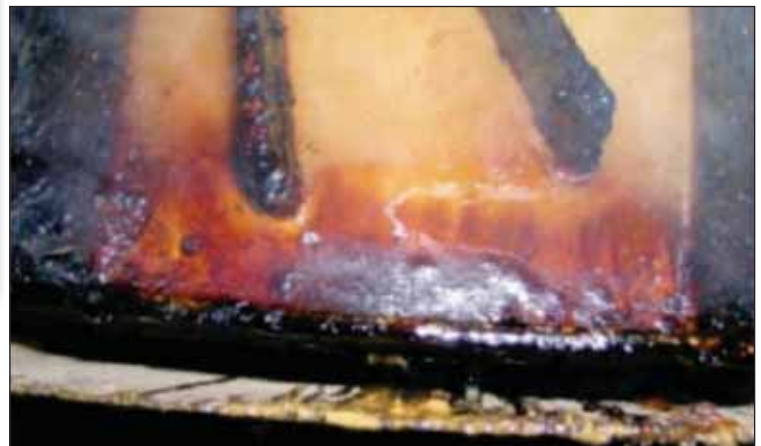
Figure 9: Glue quantity in the cylinder is too small, resulting in overheating.
