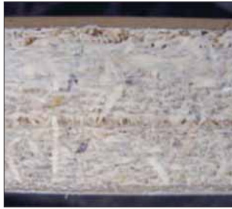
Figure 4: Lack of adhesive.
