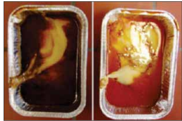
Figure 8: Comparison between EVA and PP hot-melt adhesives within eight hours after heated at 200°C
