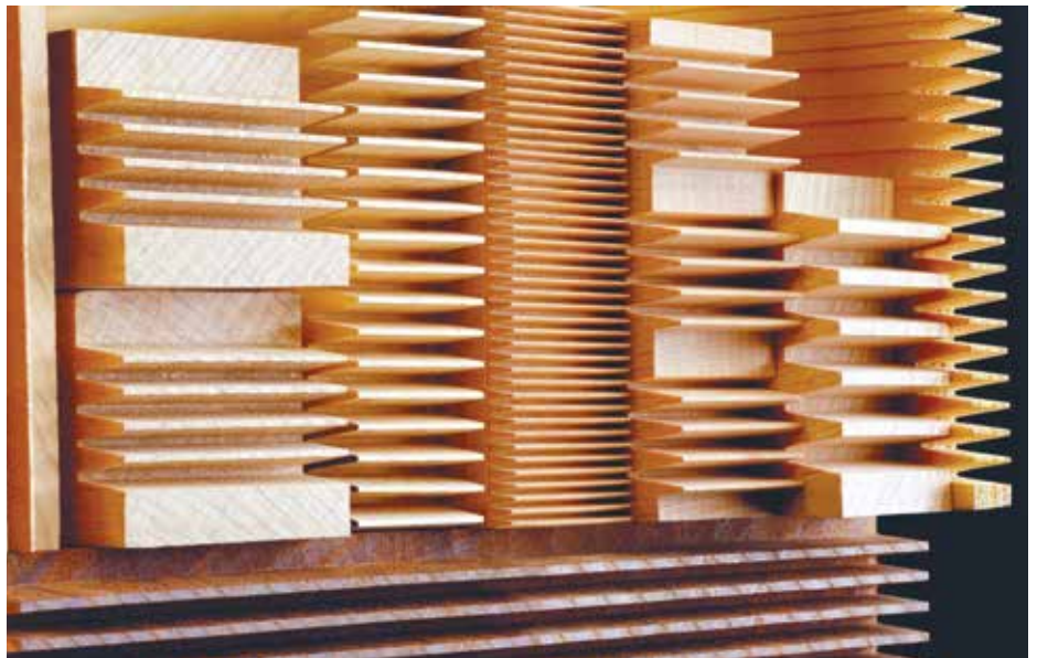
Finger jointing results in higher quality material and stronger connections between pieces and components, while also dramatically reducing waste.
