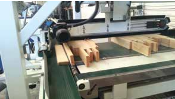
Motors directly driving the spindles transmit their vibrations to the cutters, resulting in inaccurate finger shapes and low quality products.
