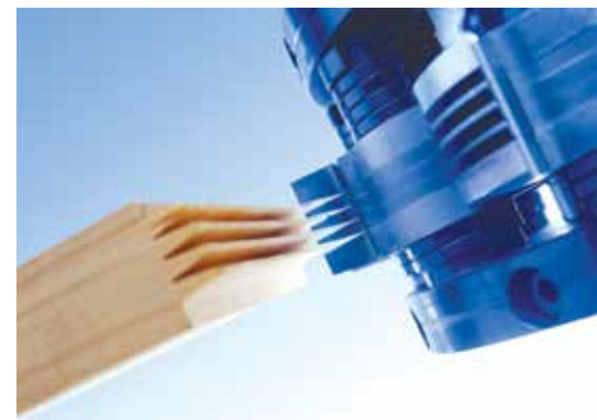
Extremely short finger length results in enormous timber saving and higher profit margins.
